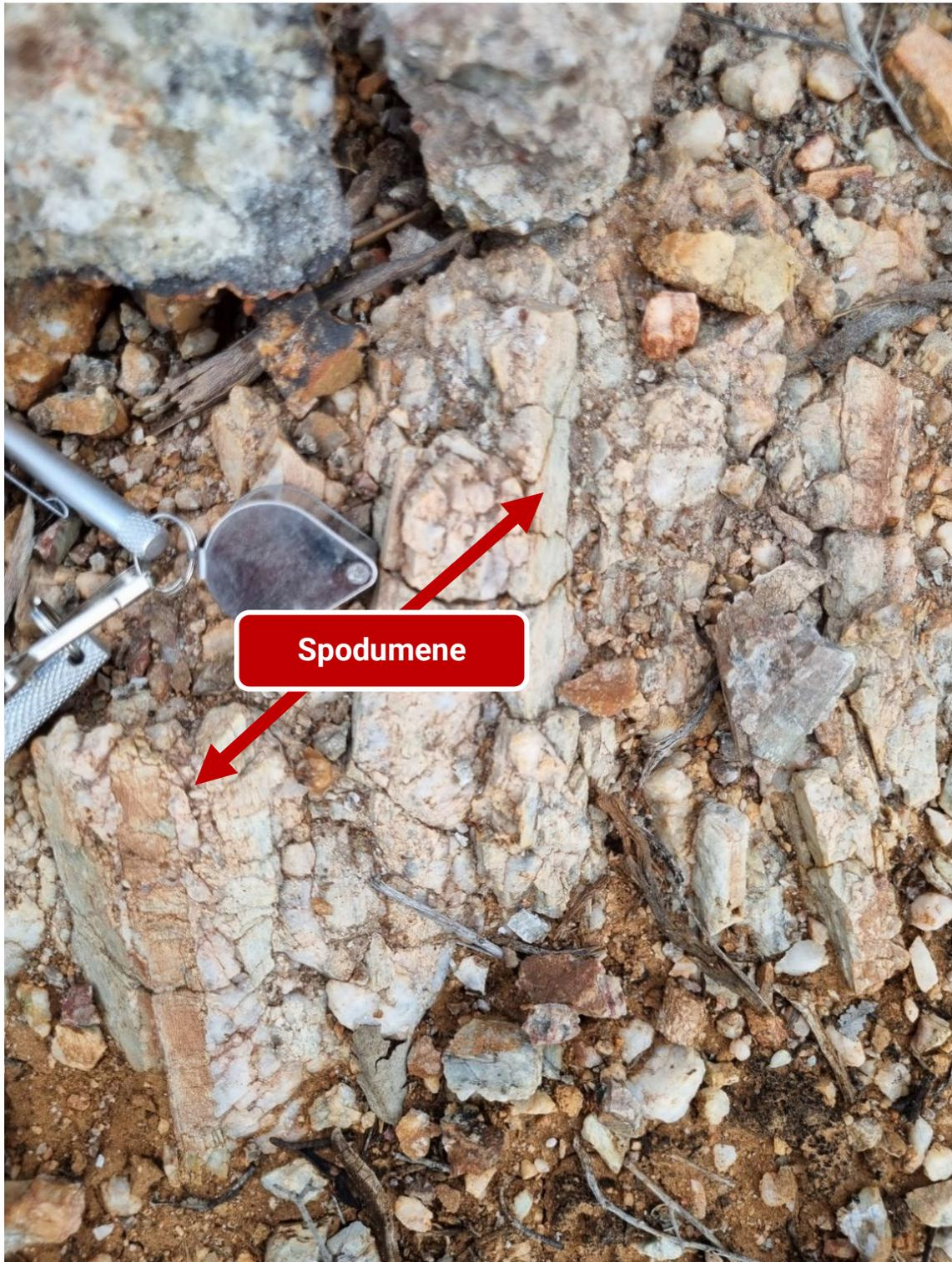
Figure 3. – Faraday prospect showing spodumene bearing pegmatite outcrop (360630mE, 6515782mN)
